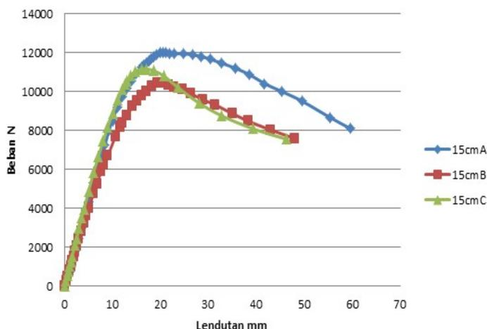
Figure 1. Graph load relations – remote Flextural Pegs 15 cm
