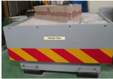
Figure 2. Vibration technique for solidification process
