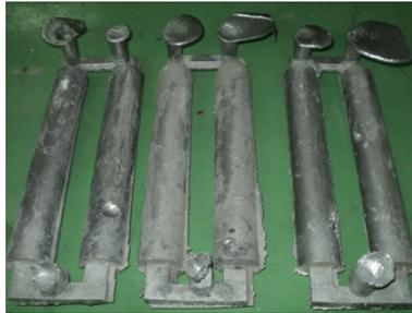
Figure 3. The round bar casting products of LM6 aluminum reinforced with 10 wt.% TiC particles.
