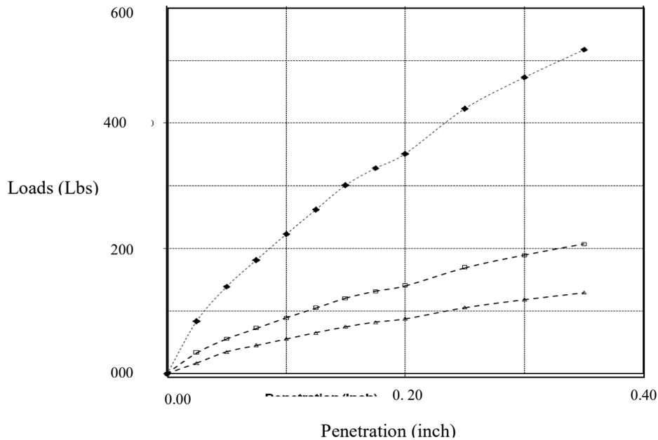
Figure3. CBR Laboratory value and load–penetration relationships
