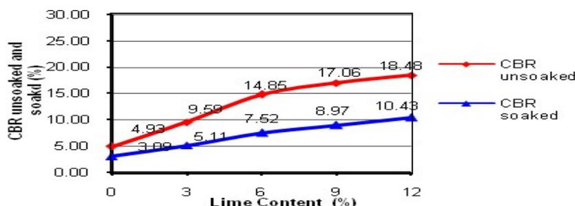
Figure 8. Correlation between CBR value with the addition of lime
