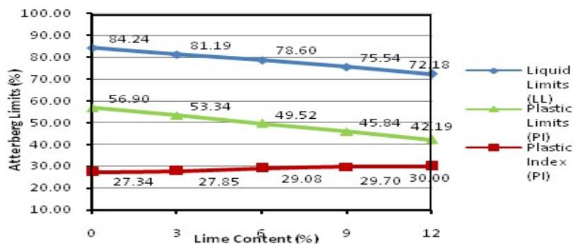
Figure 7. Correlation between Liquid Limit and Plastic Limit by the addition of lime
