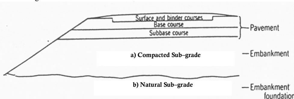
Figure 1. Type of embankment sub–grades, a) natural sub–grade and b) compacted sub–grade
