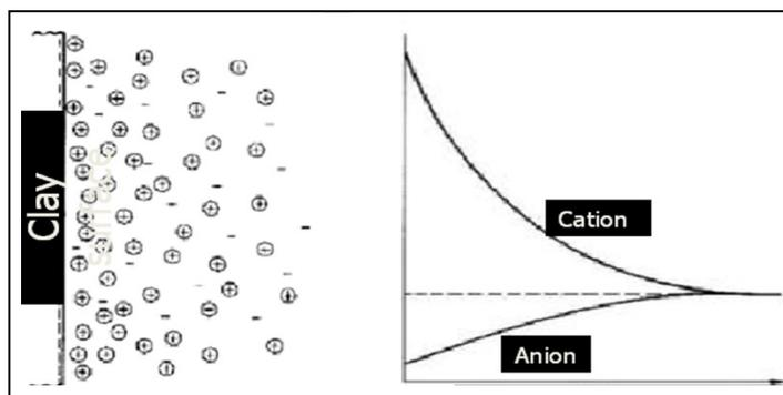
Figure2. Interaction between clay and ion of the water Physical properties of aggregate
