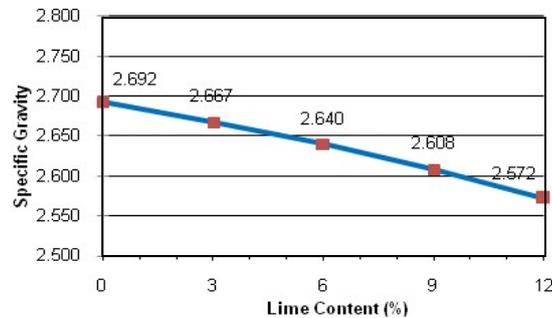
Figure 6. Correlation between Soil Specific Gravity and Level of Lime
