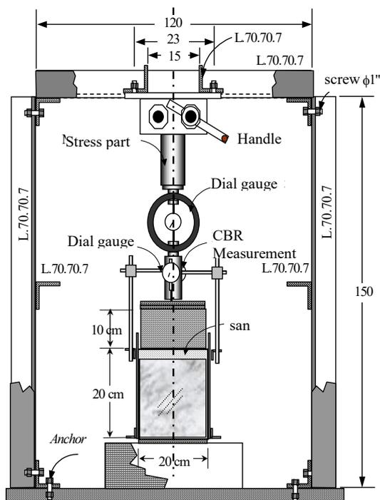
Figure 4. CBR laboratory equipment
